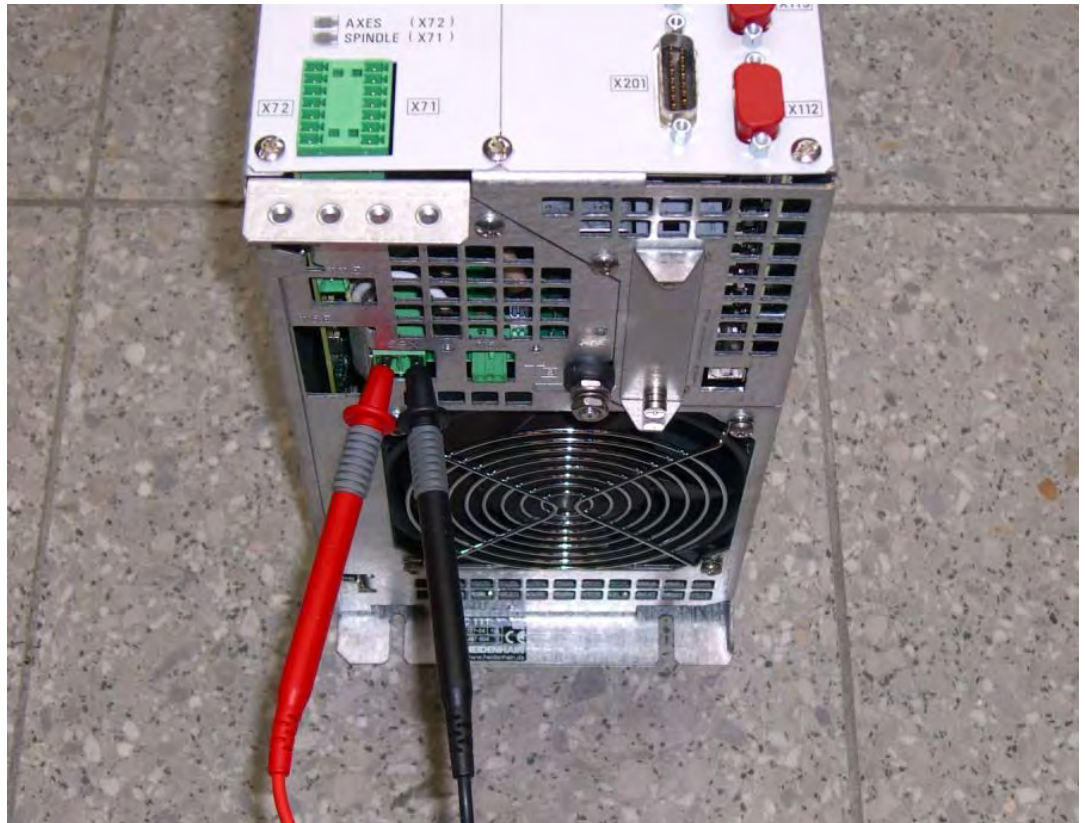
Figure: Measurement of internal braking resistor
