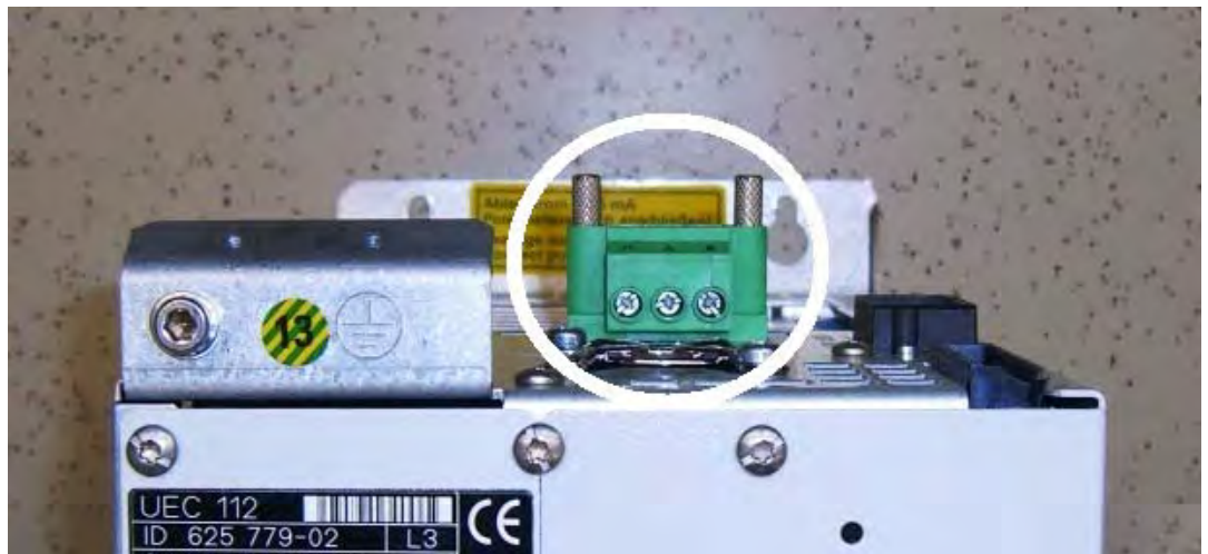
Figure: Primary voltage connection on UEC
