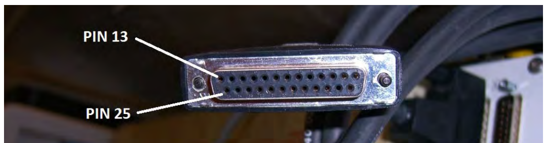
Photo: Measurement of the temperature sensor on the D-sub connector of the motor encoder cable
