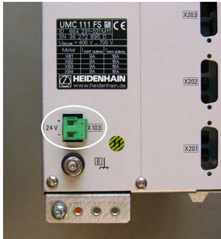
Figure: 24 V connection on the UMC
