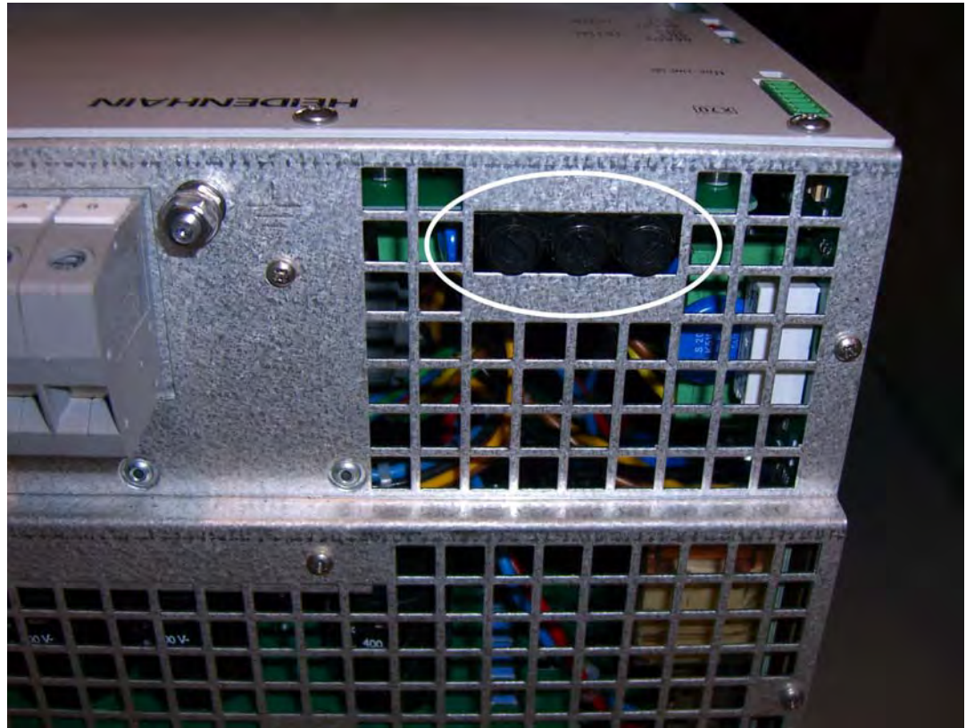
Photo: Location of the fuses
