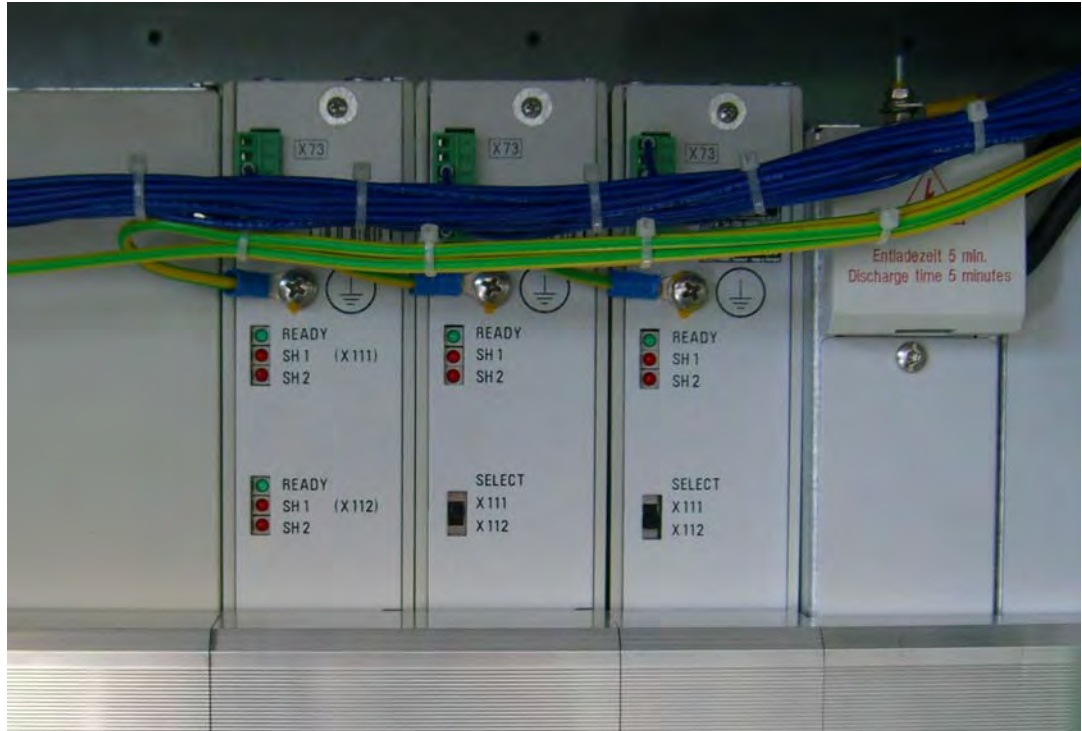
Photo: LEDs on the HEIDENHAIN expansion boards
