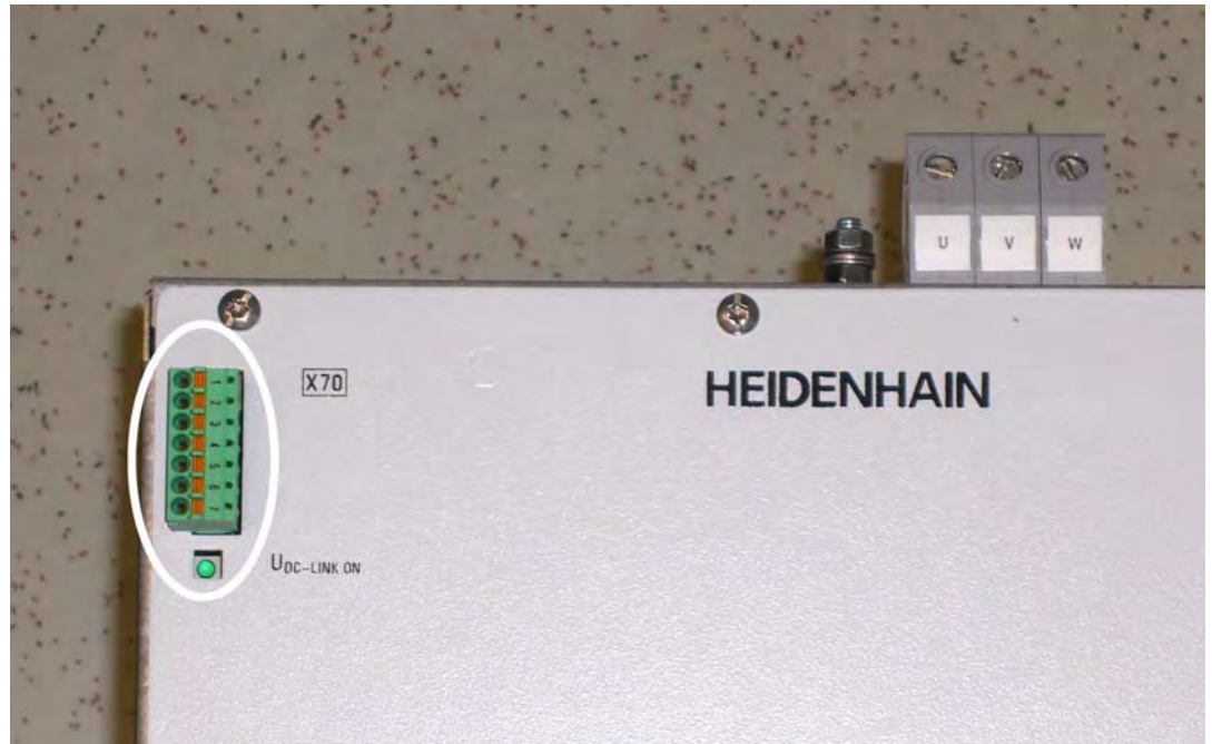
Figure: Connector X70 on the UE 241 B compact inverter
