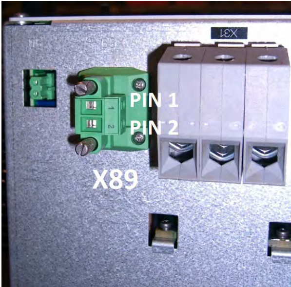
Figure: UV 130, assignment of X89
