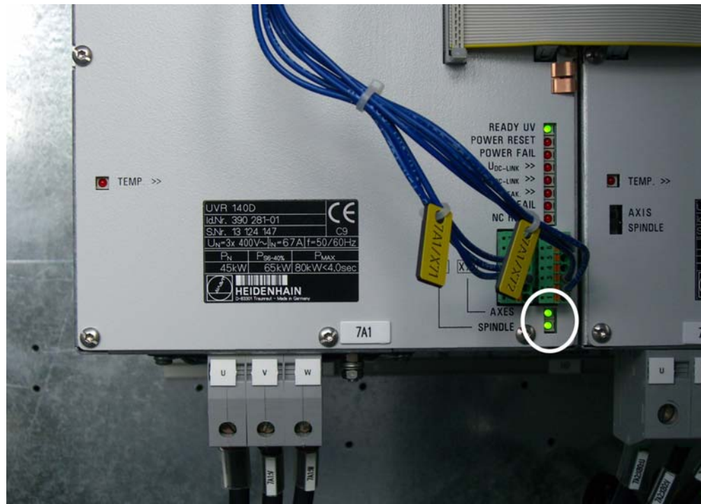
Photo: LEDs for axis and spindle enable on the UVR 140 D power supply unit
