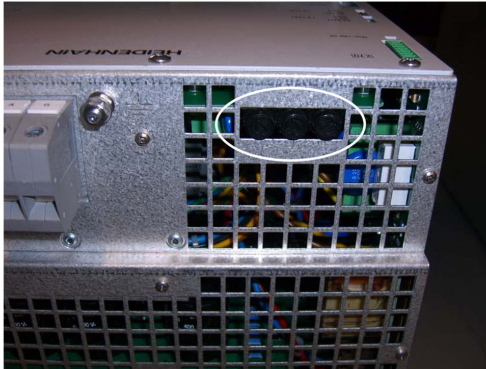
Photo: Location of the fuses
