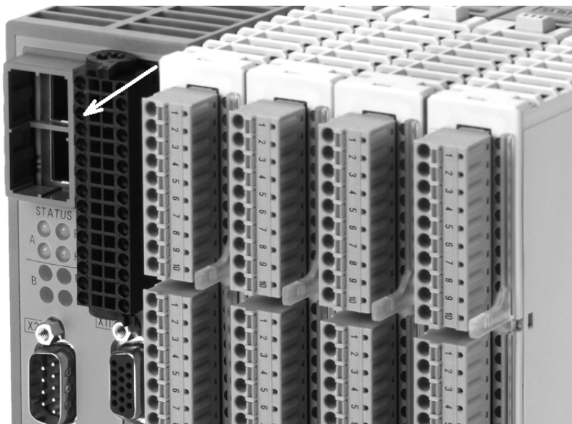
Figure: The level can be measured at the terminal RO X9.3a.
