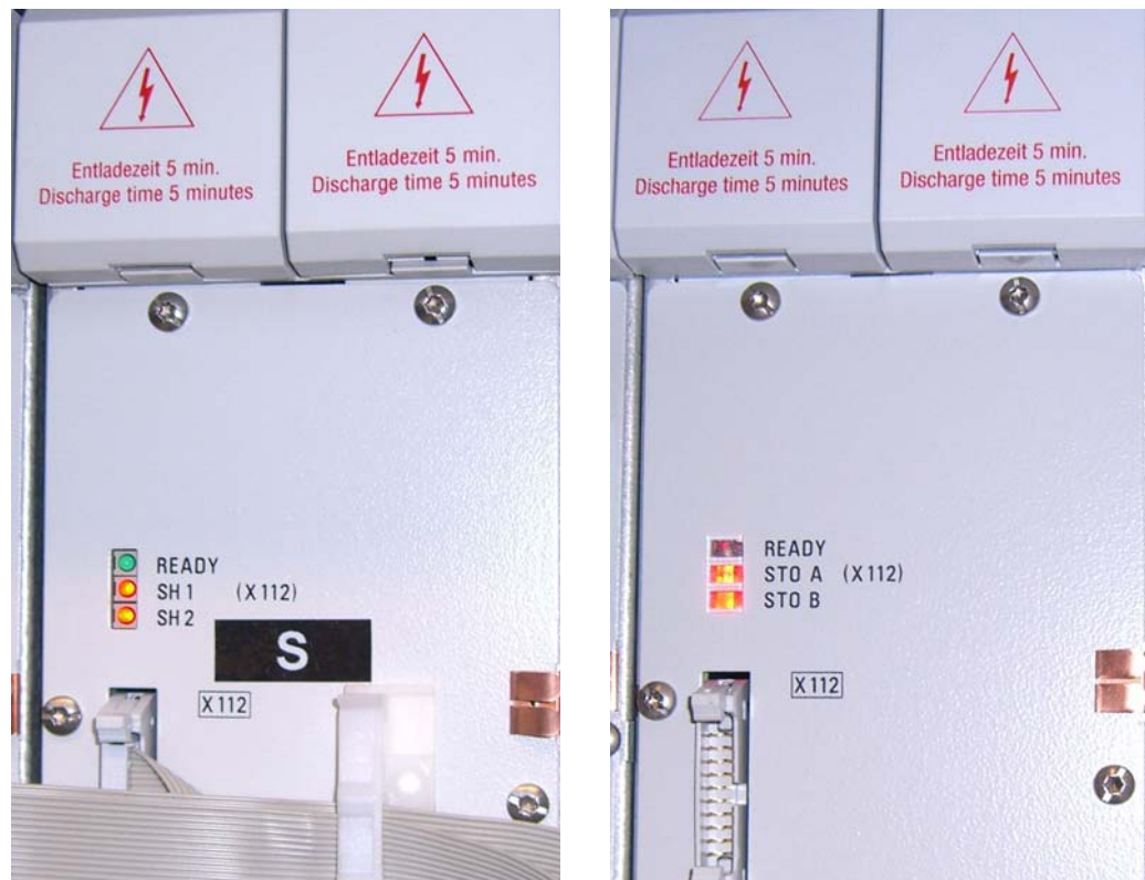
Figure: LEDs SH 1 / SH 2 and STO A / STO B on HEIDENHAIN UM units
