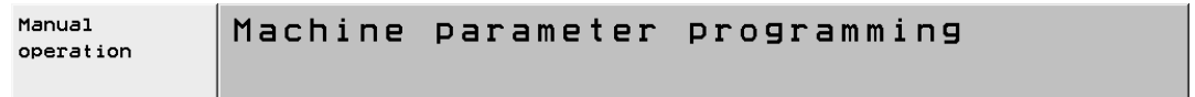
Figure: As long as the text Machine parameter programming is displayed in the header, no further code numbers are accepted (exception: NET123).
