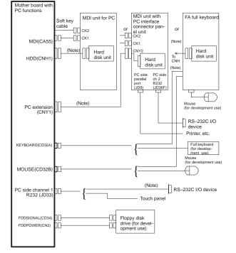
The following figure shows the specific connection to the Series 160*i*/180*i* control unit having PC functions.
