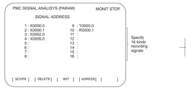
(a) [SCOPE] soft key : Select the signal wave display screen.
