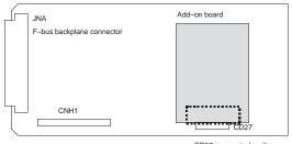
CD27 is mounted on the add-on board.
