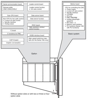
On a unit with two option slots, two option boards can be mounted. On a unit with three option slots, three option boards can be mounted. On a unit with four option slots, iour option boards can be mounted. (On the unit with four option slots, just a data server board or HSSB interface board can be fit into the slot furthest from the LCD.)
