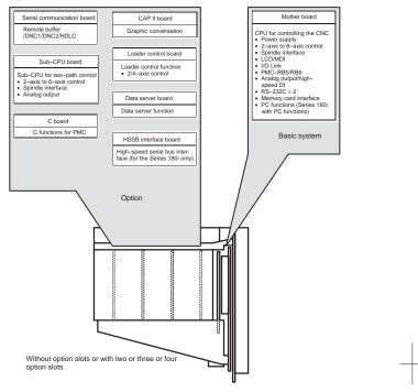
On a unit with two option slots, two option boards can be mounted. On a unit with three option slots, three option boards can be mounted. On a unit with four option slots, four option boards can be mounted. (On the unit with four option slots, just a data server board or HSSB interface board can be fit into the slot furthest from the LCD.)
