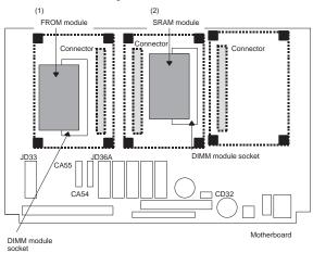
No. Name Specification Function Remarks (1) FROM module A20B-3900-0010 CNC system 16M Servo system A20B-3900-0011 12M A20B-3900-0012 8M A20B-3900-0013 6M A20B-3900-0014 4M A20B-3900-0015 2M (2) SRAM module A20B-3900-0020 SRAM for the ЗM system A20B-3900-0060 2M 7 A20B-3900-0061 1M A20B-3900-0052 512K A20B-3900-0053 256K
