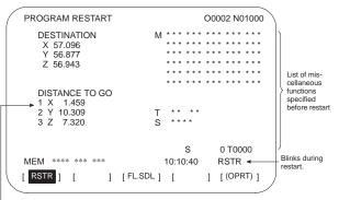
Axis sequence set in parameter No. 7310 (Displays \* when the preparation for restart is not completed. Displays the axis sequence when searching the restarting block is completed. Blinks when the preparation is completed.)
