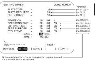
NOTE \*1 Cannot be changed on this screen (but can be changed on the parameter screen).)
