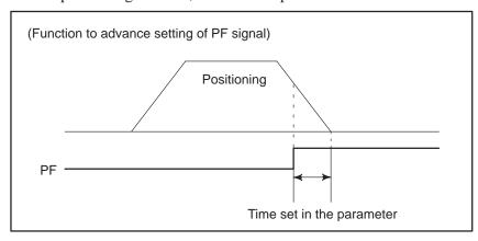
If the time set here is longer than the time required for deceleration, the PF signal is set to 1 when deceleration starts.
