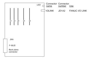
Fig. 7.4.5 (a) Parts Layout of the Option 3 Board
