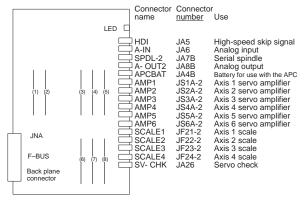
Fig. 7.4.4 (a) Parts Layout of the Option 2 board for Series 16
