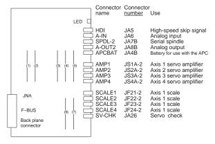
Fig. 7.4.4 (b) Parts Layout of the Option 2 board for Series 18
