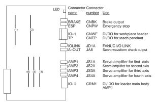
Fig. 7.4.6 (a) Parts Layout of the Loader Control Board
