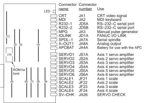
Fig. 7.4.2 Parts Layout for the Main CPU Board
