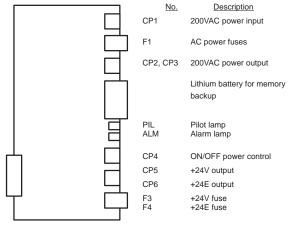
Fig. 7.4.1 Power Unit Parts Layout
