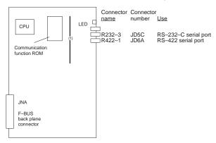
Fig. 7.4.3 (a) Parts Layout for the Option 1 Board
