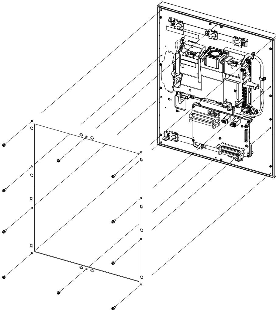
Fixing screw: Use M4×10 with spring washer and plain washer (10 screws).
