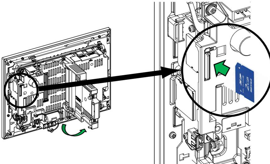
(Note 1) Do not eject an SD card during the data reading/writing.
