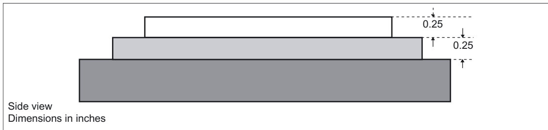
Dimension drawing of workpiece "The Raised Boss" (not to scale).
