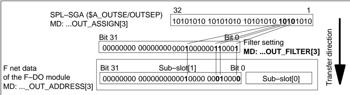
Fig. 5-47 Filtering the SPL-SGA in the output direction
