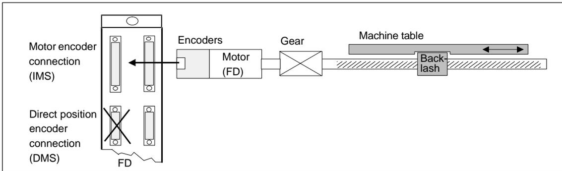
Fig. 4-1 1-encoder system for a feed drive (FD)
