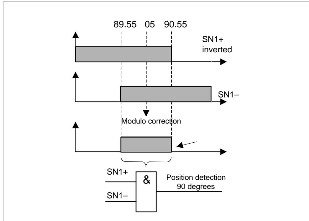
Fig. 10-50 Negating an SN signal to generate a pulse
