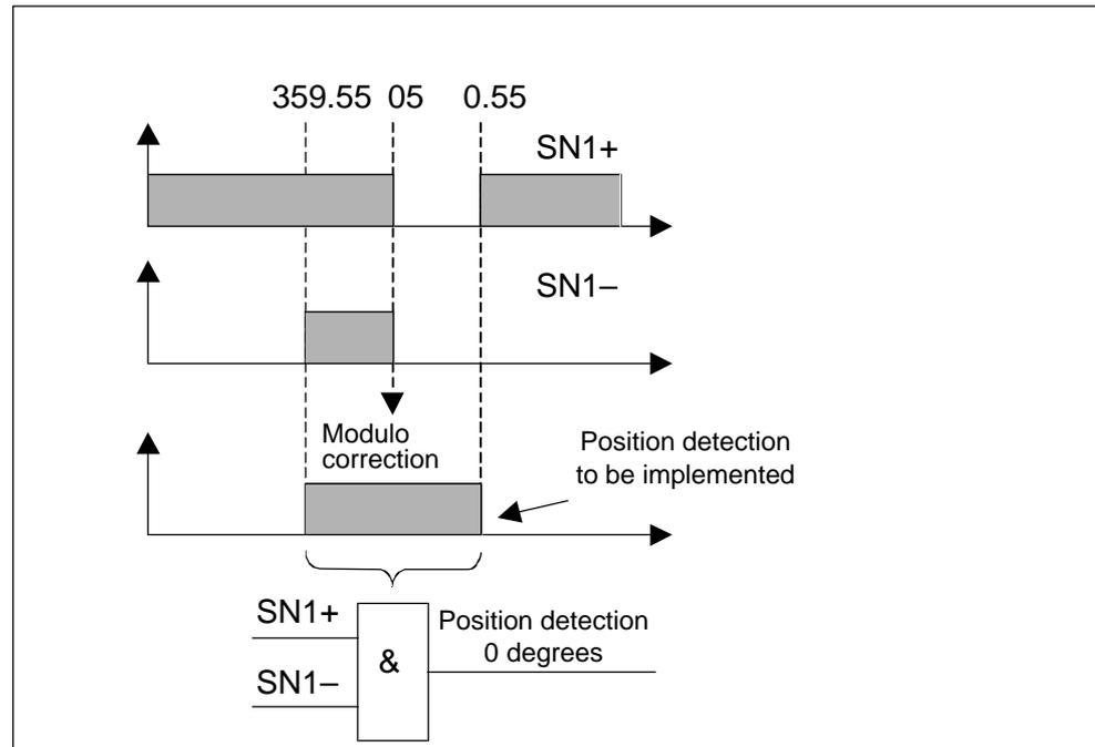
Fig. 10-51 Signal generator for modulo cam 1
