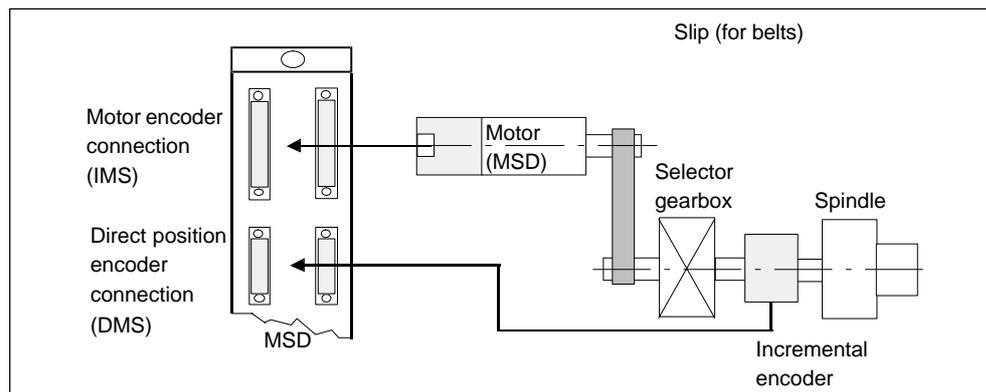
Fig. 10-58 Motor for a drive subject to slip
