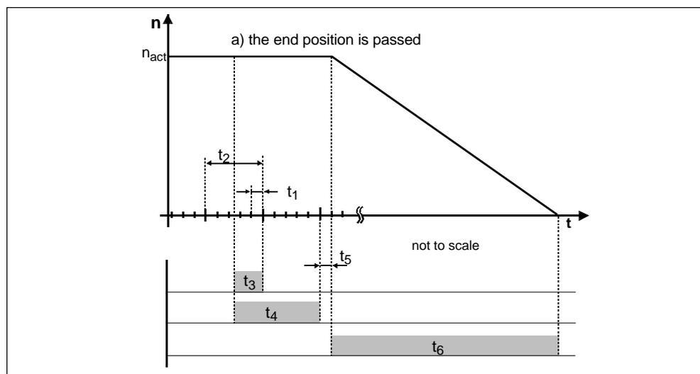
Fig. 5-17 Timing when a software limit switch is actuated
