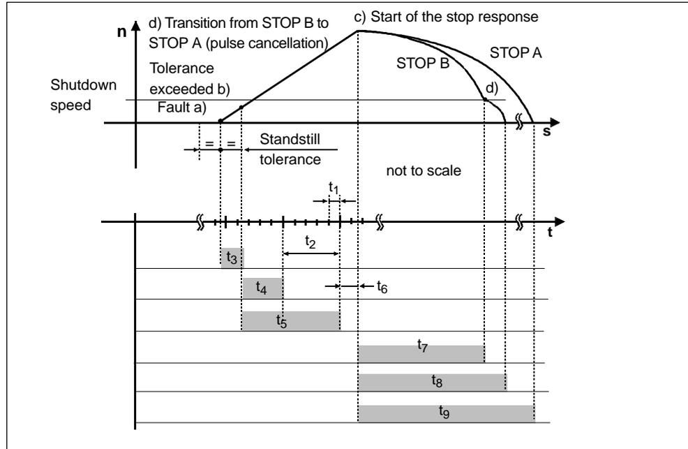
Fig. 5-14 Timing when the limit value is exceeded for SBH
