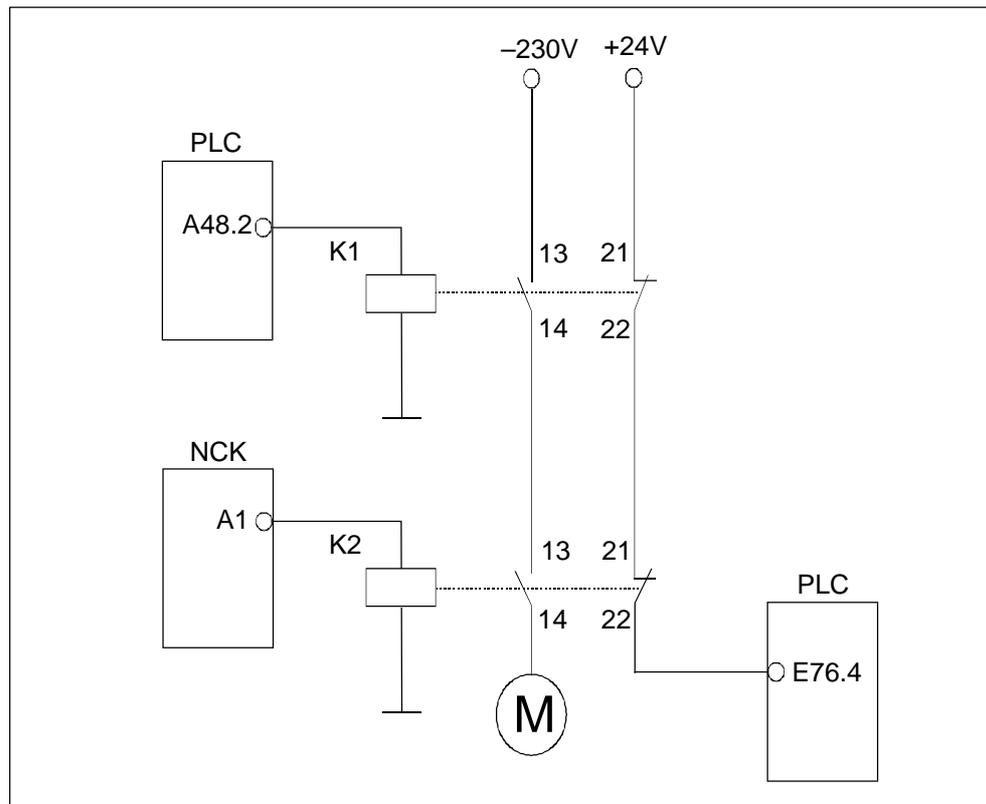
Fig. 10-8 Circuit diagram
