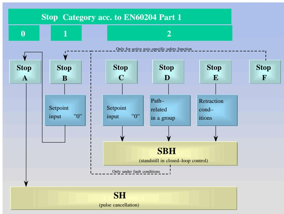
Fig. 5-7 Stop responses, safe operating stop (SBH), safe standstill (SH)
