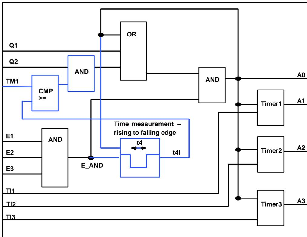
Fig. 5-33 Function diagram of the "safety relay"
