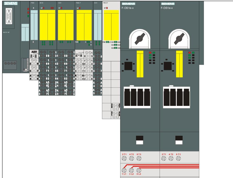
Fig. 10-30 Design and structure of the DP slave
