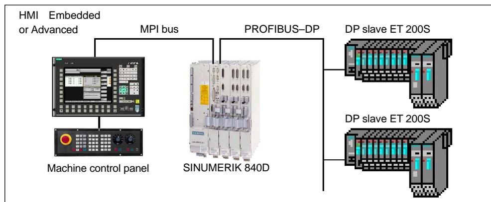
Fig. 5-37 SI I/Os using fail-safe modules connected to PROFIBUS-DP
