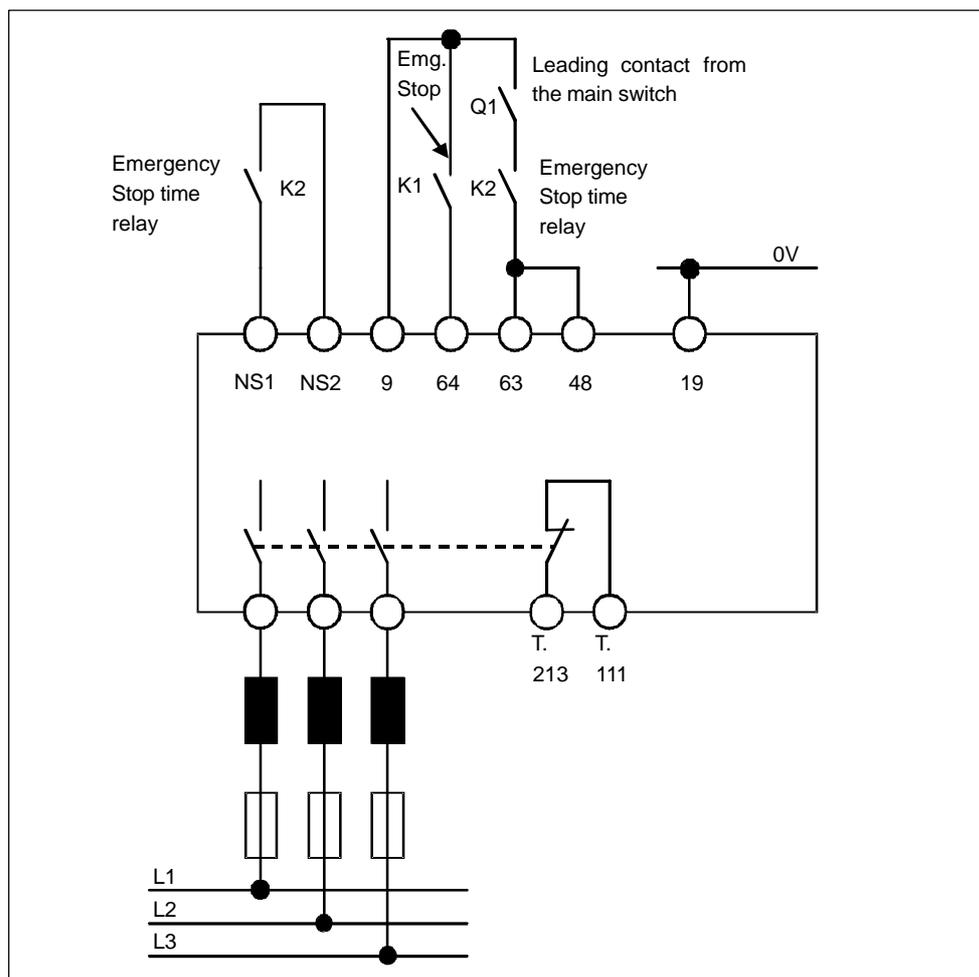
Fig. 10-23 Connecting-up the infeed/regenerative feedback module without SPL
