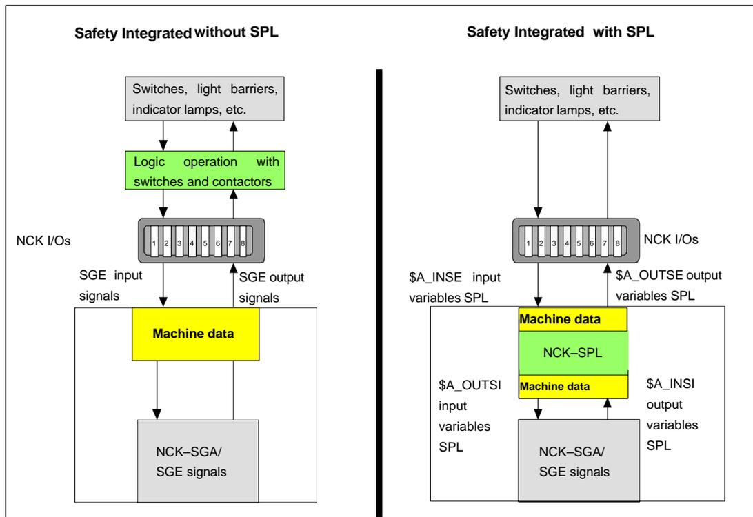
Fig. 10-21 Function schematic of SI without SPL
