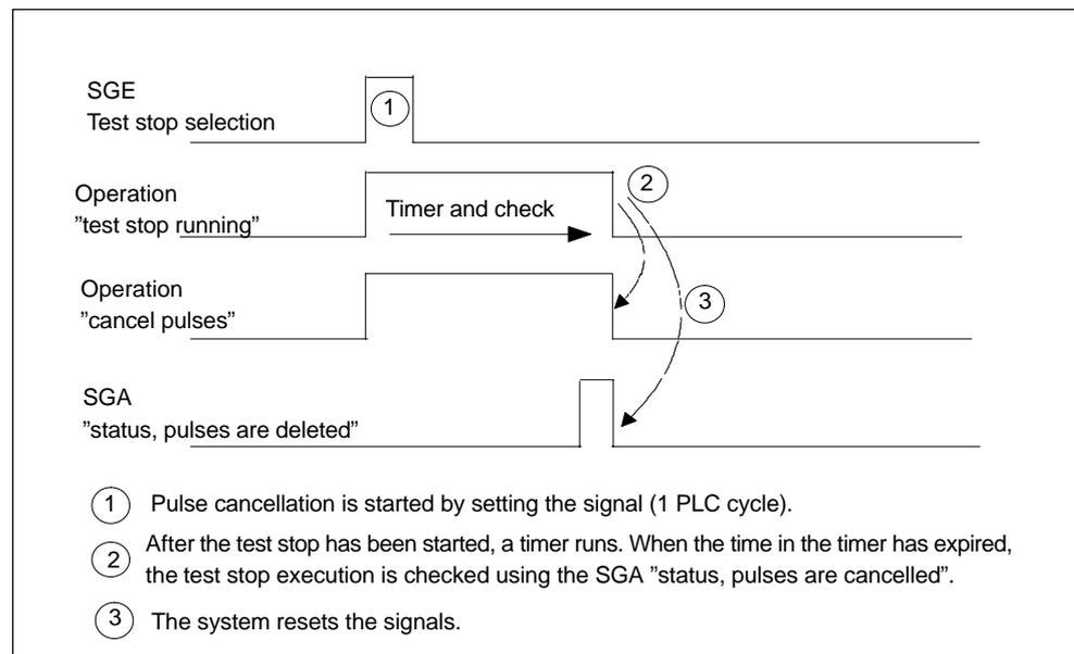
Fig. 6-1 Signal timing for SGE test stop selection
