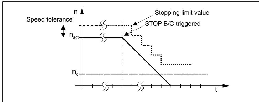
Fig. 5-22 Characteristics of the stopping limit value for SBR
