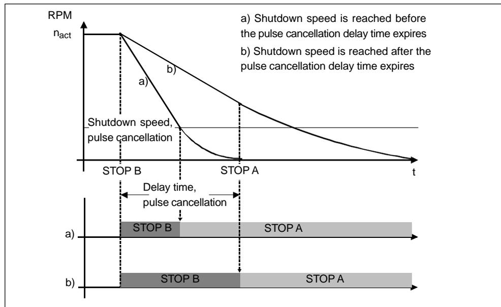
Fig. 5-8 Transition from STOP B to STOP A
