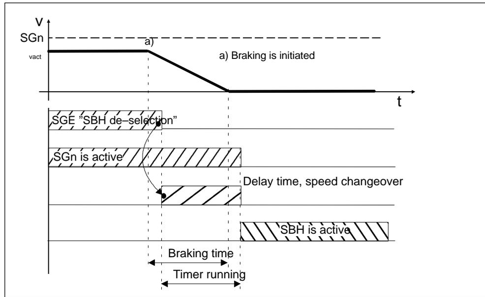
Fig. 5-13 Timing when SBH is selected from SG
