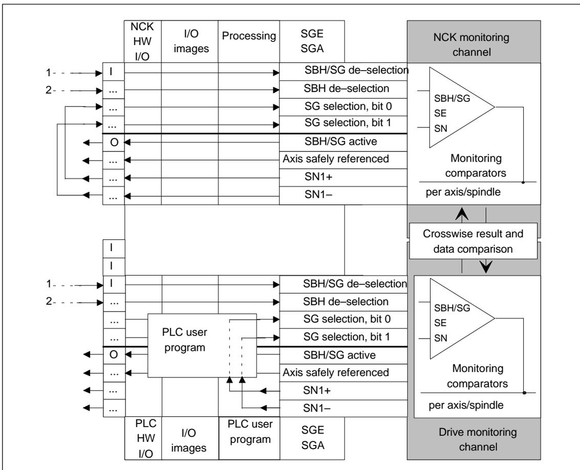
Fig. 5-21 Connecting the required SGEs/SGAs (without SPL)
