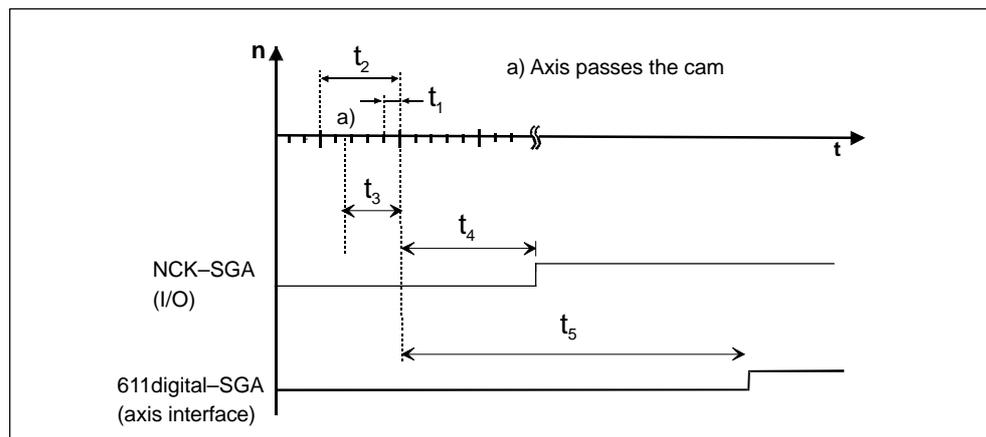
Fig. 5-19 Timing when the cam position is passed
