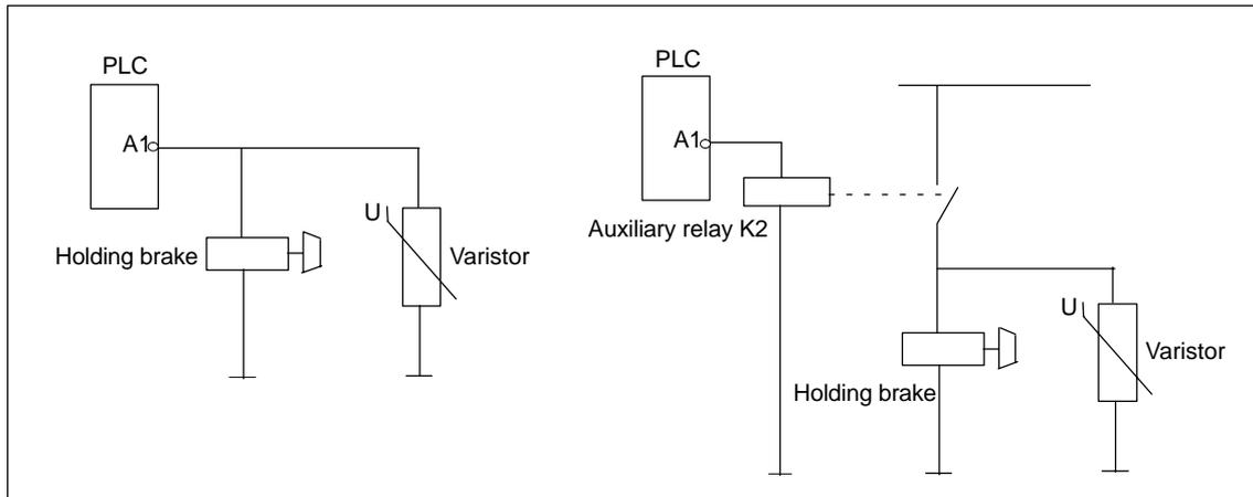
Fig. 10-43 Single-channel brake control, P-switching (single-channel from the PLC)
