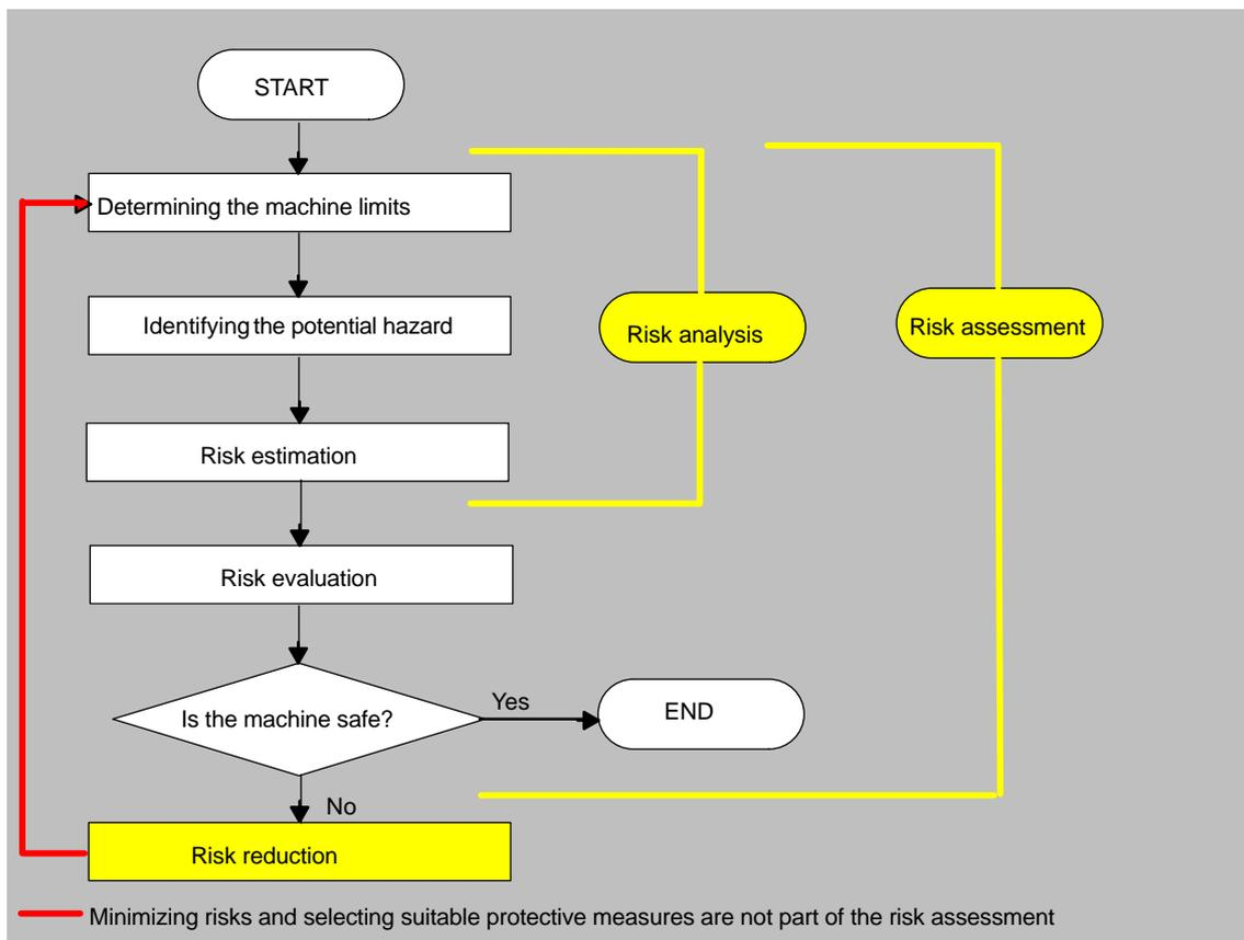
Fig. 1-1 Iterative process to achieve safety in compliance with ISO 14121 (EN 1050)
