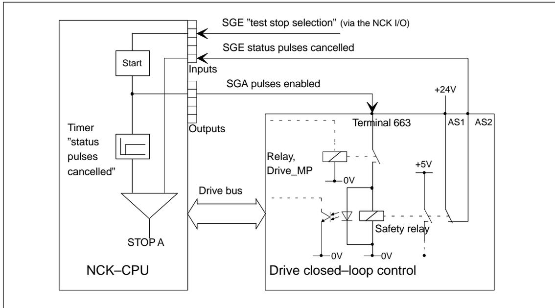
Fig. 5-3 Shutdown path of the NCK-CPU using terminal 663
