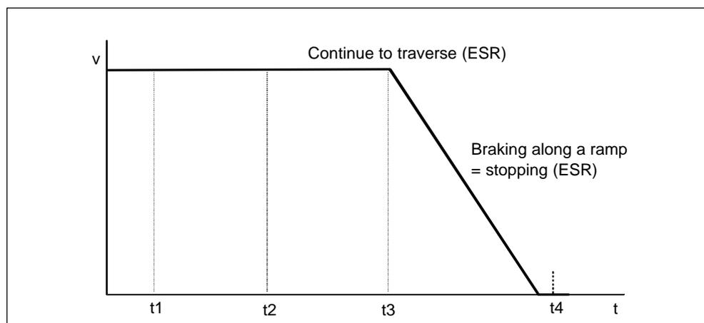
Fig. 5-10 Velocity characteristic of an SI axis when stopping with STOP F
