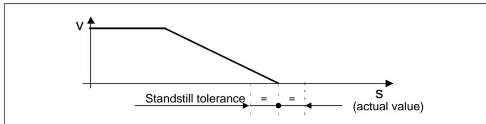
Fig. 5-12 Standstill tolerance
