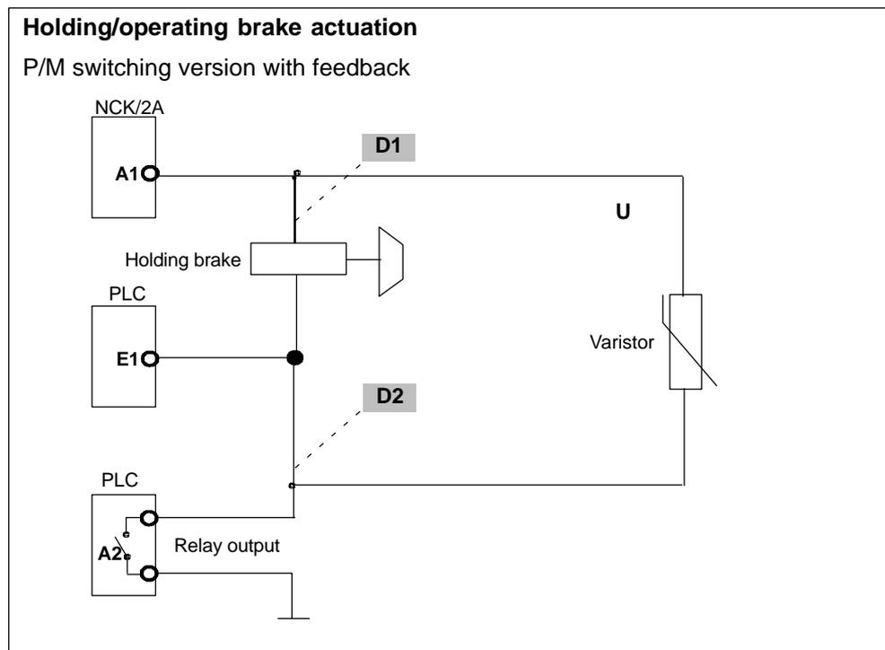
Fig. 10-44 Two-channel brake control, P/M switching with SI
