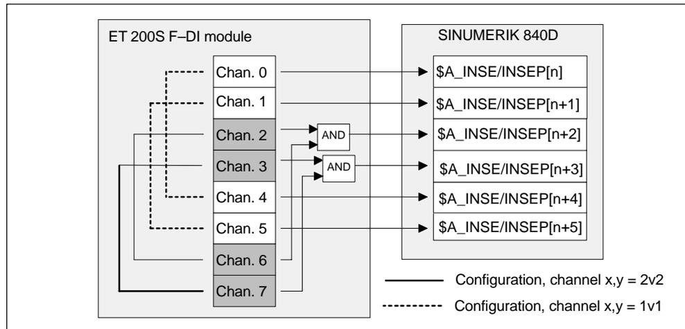
Fig. 5-40 2v2/1v1 mapping of the F-DI channels to SPL input data
