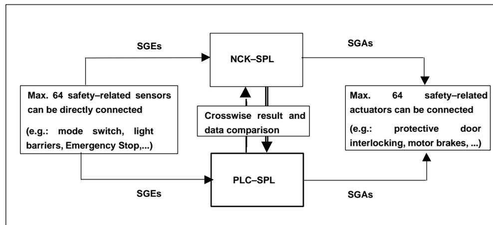
Fig. 5-30 Safe programmable logic
