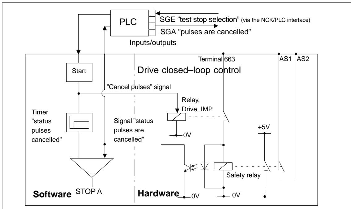
Fig. 5-2 Shutdown paths of the drive CPU
