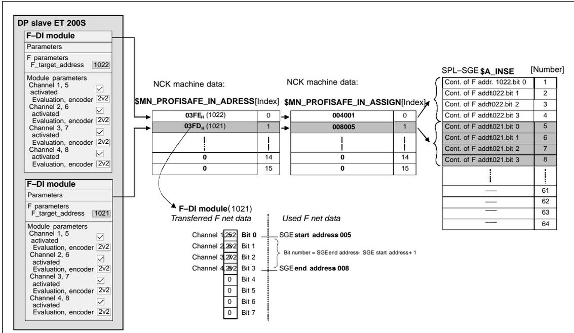
Fig. 5-42 Assignment example: F net data to SPL-SGEs
