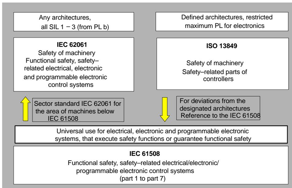
The areas of application of ISO 13849-1 and IEC 62061 are very similar. In order to help users make a decision, the IEC and ISO associations have defined in detail the application areas of both Standards in a common table in the introduction to the Standards. Either EN ISO 13849-1 or EN IEC 62061 is applied depending on the particular technology (mechanical, hydraulic, pneumatic, electrical, electronic, programmable electronic), risk classification and architecture.
