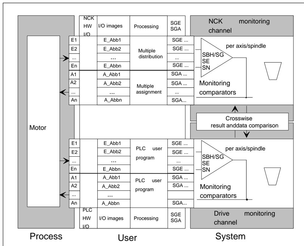
Fig. 5-26 I/O signal processing through two channels
