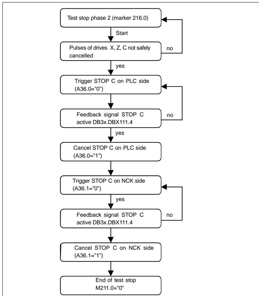
Fig. 10-28 Flowchart when testing an external STOP C
