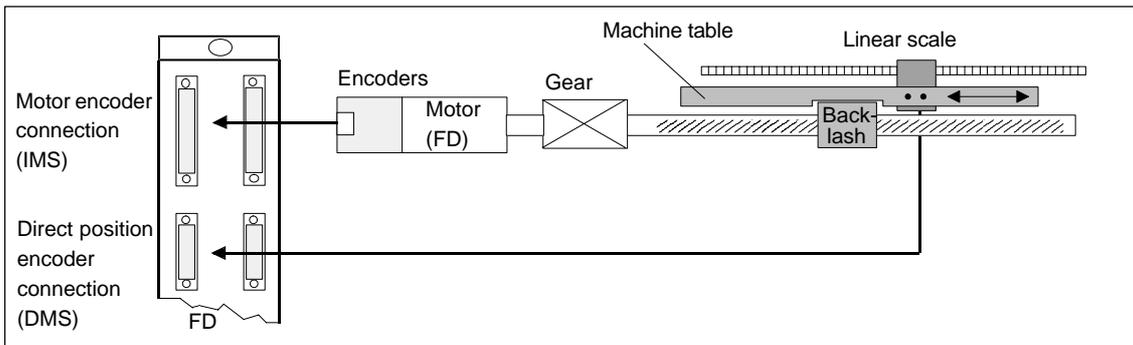
Fig. 4-2 2-encoder system for a feed drive (FD)
