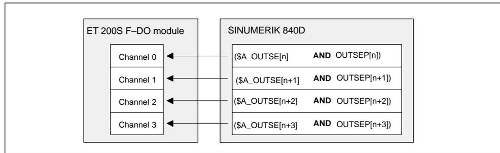
Fig. 5-41 Mapping the SPL output data to F-DO channels
