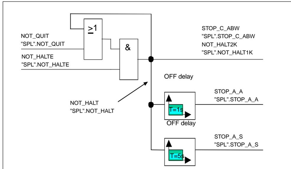
Fig. 10-10 Emergency Stop logic
