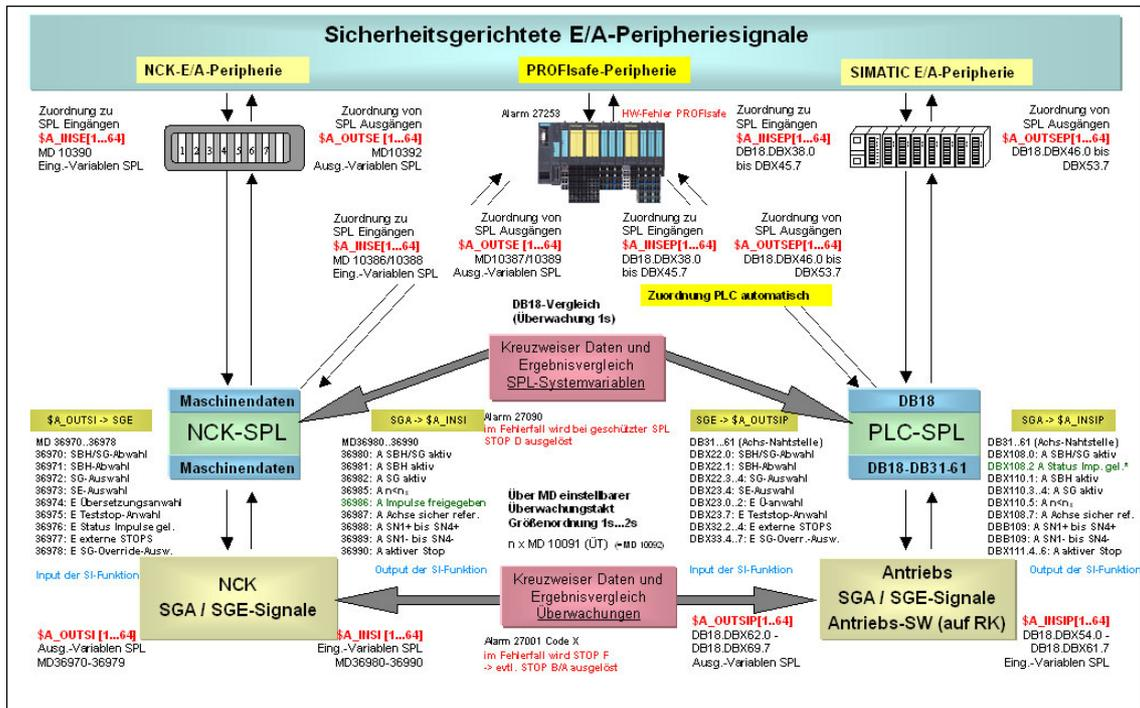
Fig. 10-3 Function chart – a detailed view of this diagram is provided in the Attachment (10.3.12)
