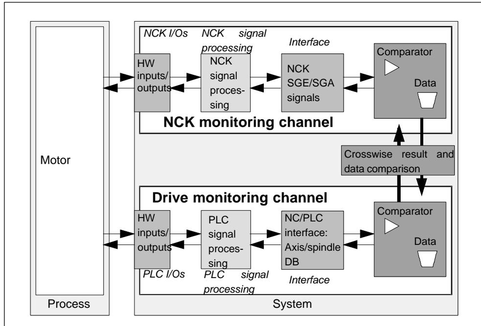
Fig. 5-31 Communications between the NCK-611 digital PLC components
