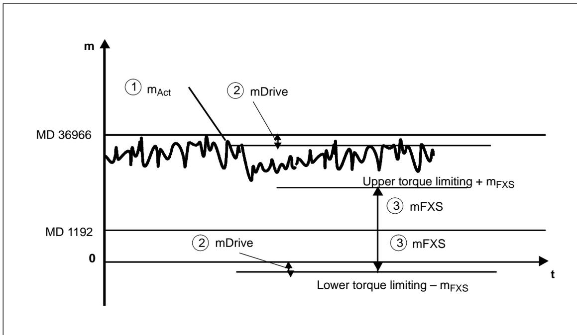
Fig. 10-48 Example of incorrect parameterization
