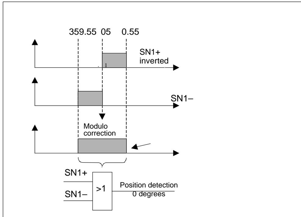
Fig. 10-52 Signal generator for modulo cam 2
