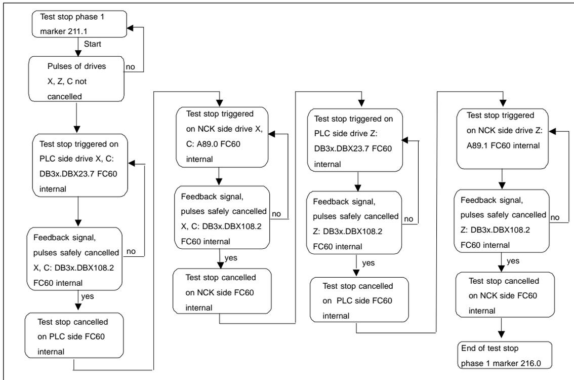
Fig. 10-12 Function diagram
