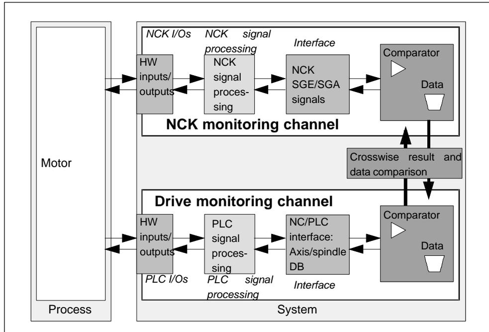
Fig. 5-25 NCK and drive monitoring channel
