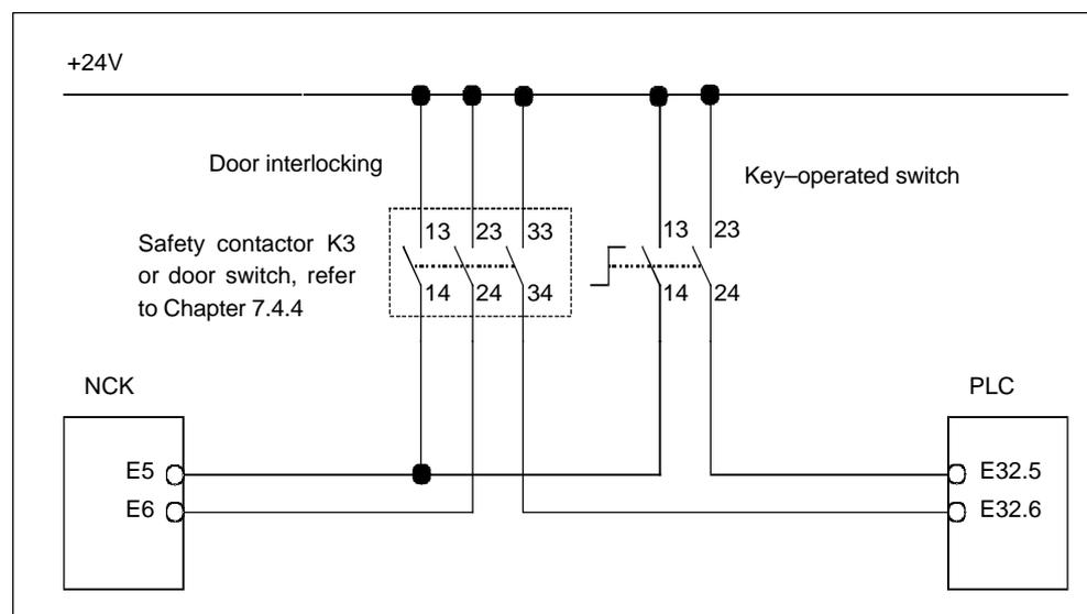
Fig. 10-27 Circuit diagram: SBH de-selection using a key-operated switch
