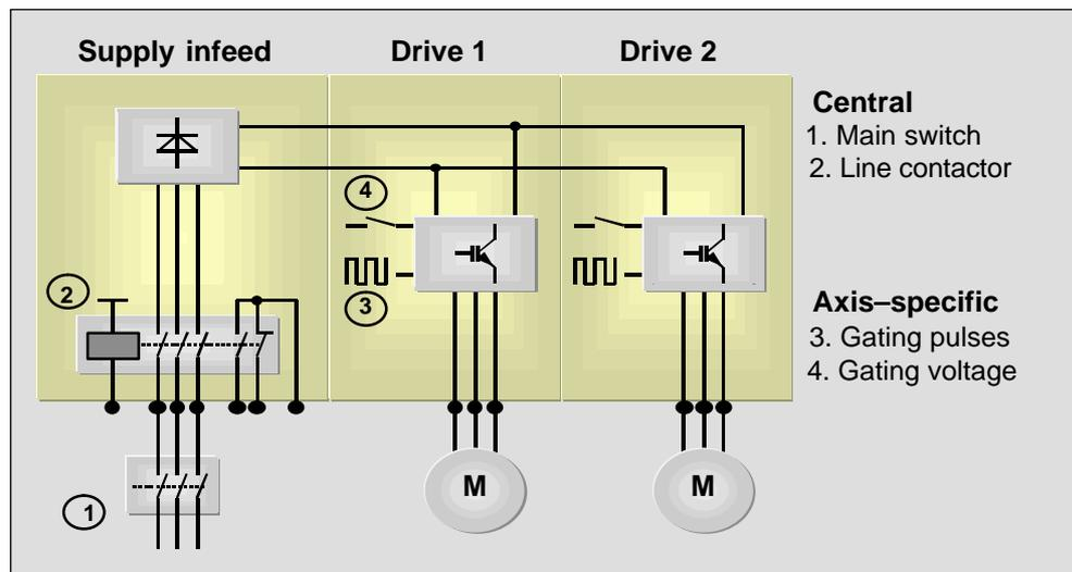
Fig. 5-1 Safe standstill – disconnecting the energy feed
