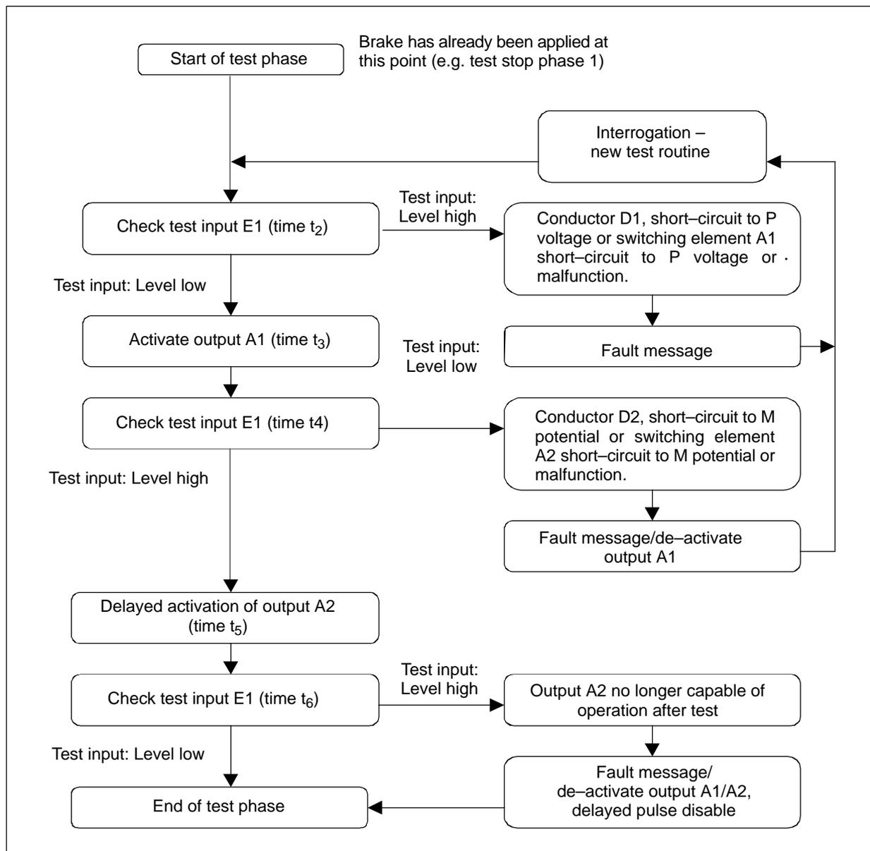
Fig. 10-46 Flowchart for the test routine
