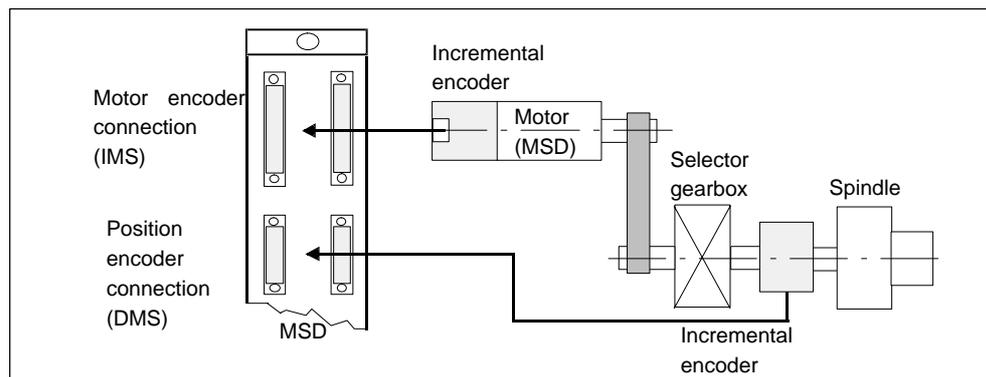
Fig. 4-3 2-encoder system for a main spindle
