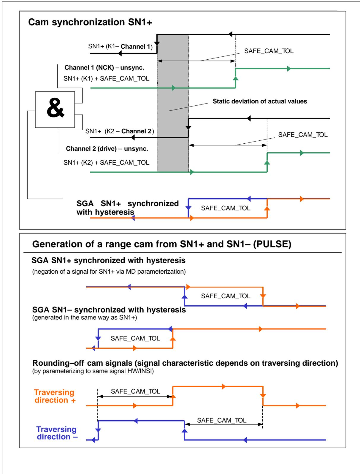
Fig. 10-54 Signal generator for modulo cam 2
