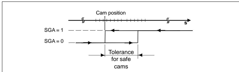
Fig. 5-18 Hysteresis of cam SGAs
