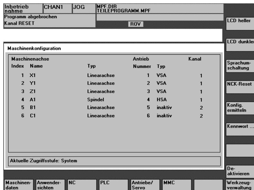
Fig. 7-1 Example of "Start-up\machine configuration" for 840D
