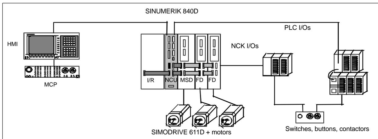
Fig. 10-2 Structure of the control and drive components
