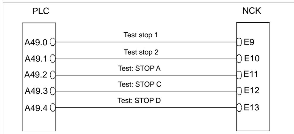
Fig. 10-11 SGE wiring to select a test stop
