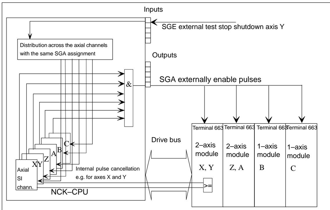
Fig. 5-5 Configuring the "test stop external shutdown"
