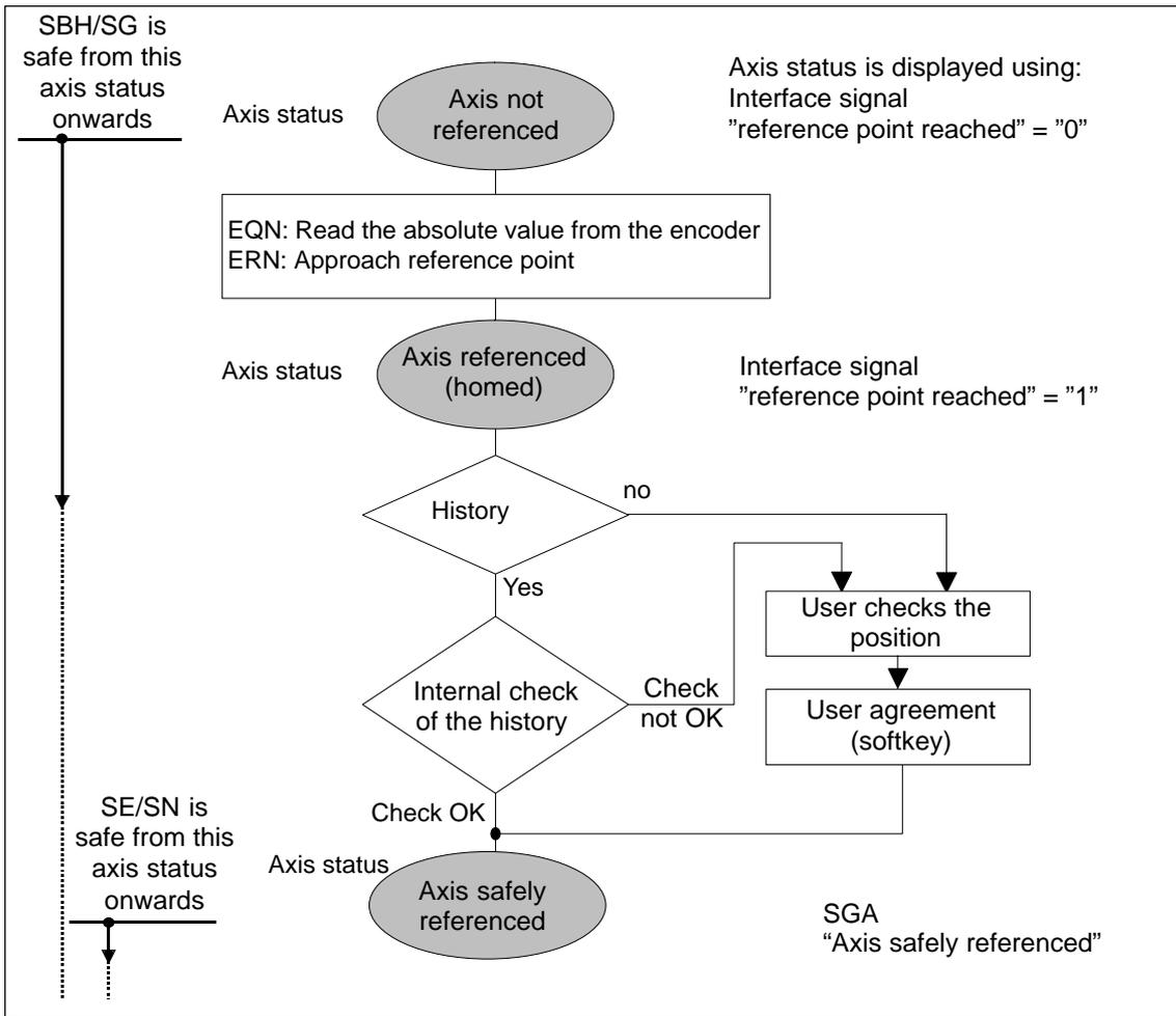
Fig. 4-5 Axis states when referencing
