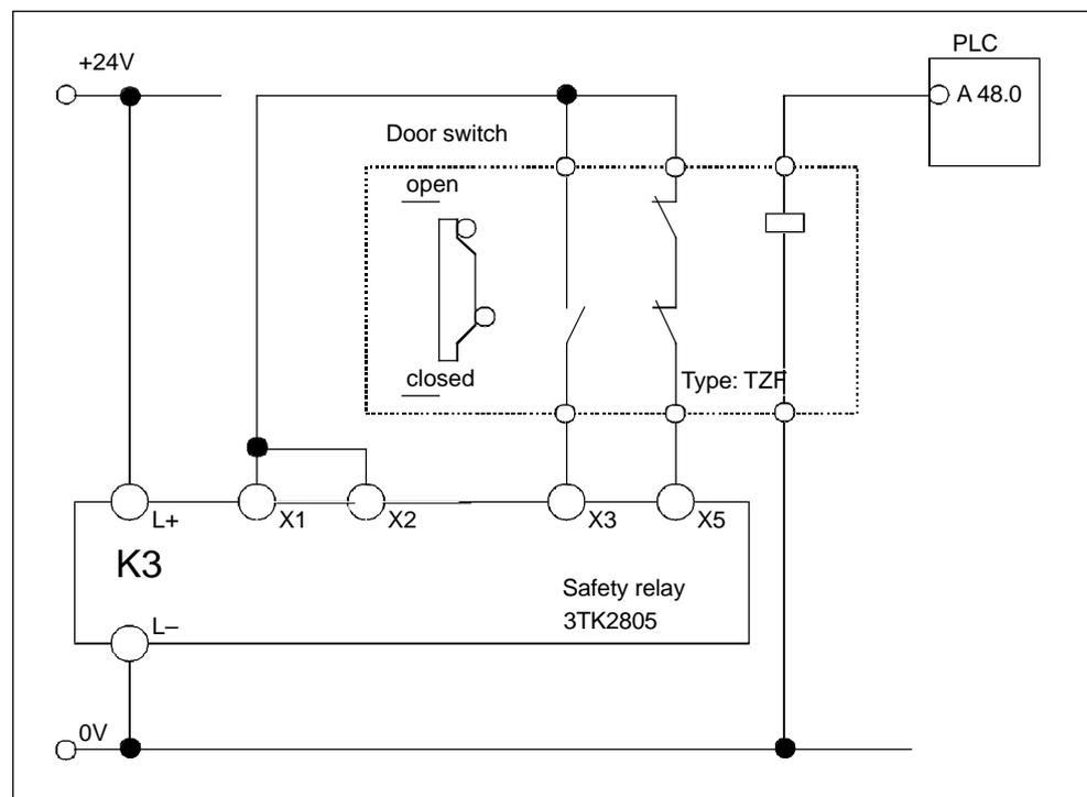
Fig. 10-26 Circuit diagram for the protective door interlocking
